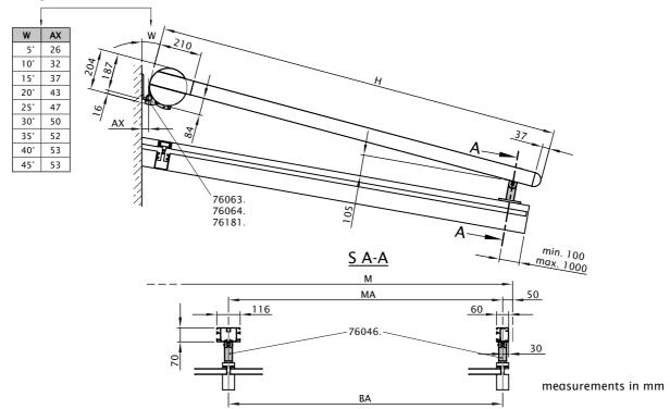
Fixture type 22, face fixture with lateral flat track bracket
