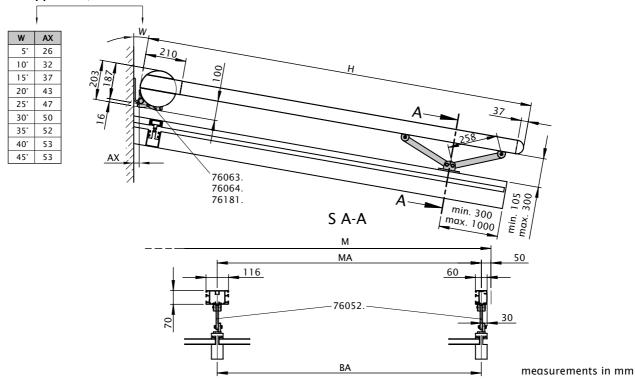
Fixture combination 51, face fixture for extensions greater than 4000 mm, up to an extension of 4000 mm fixture type 12
